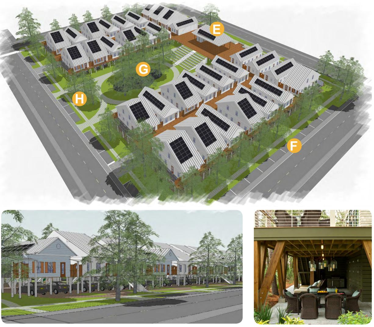
Elevated Housing in moderate-risk areas protect from flooding and provide space underneath for parking and gathering. In the model above, homes share a single elevated platform, reducing construction costs while preserving a single-family housing typology.
