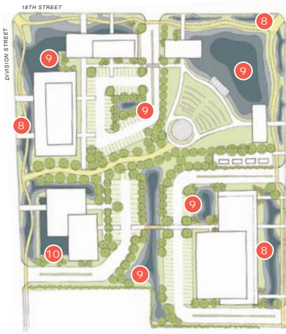
Rain Event During a rain event, bioswales and retention ponds provide stormwater storage. Elevated businesses remain accessible via boardwalks.
